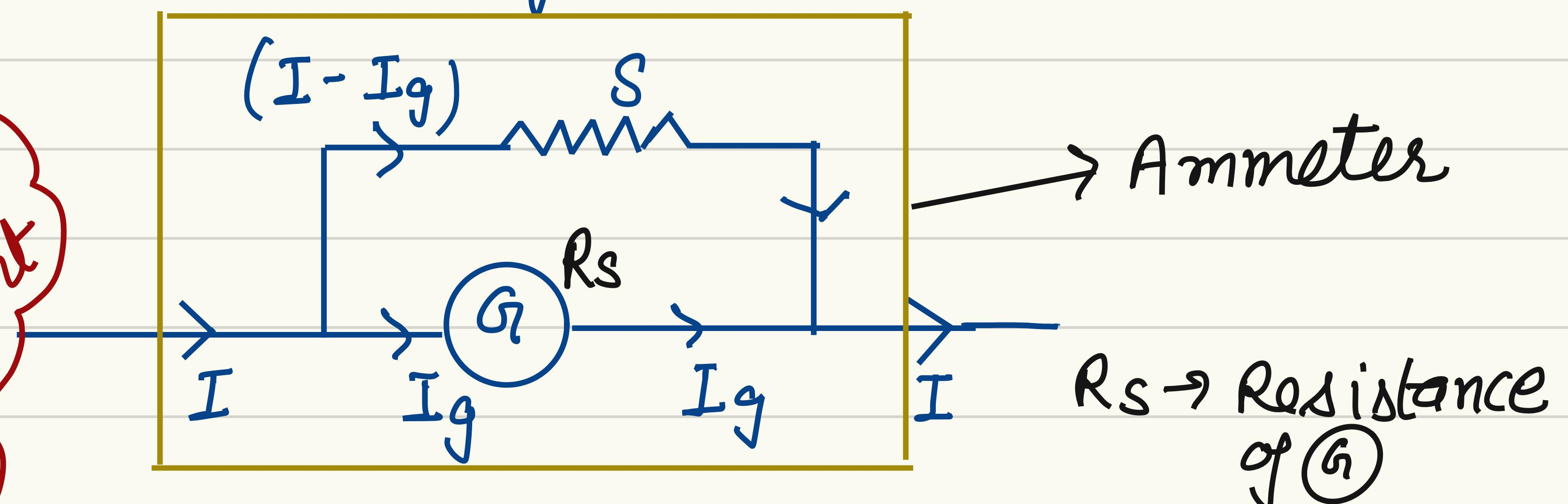
$$V_{\text{galvanometer}} = V_{\text{shunt}}$$
