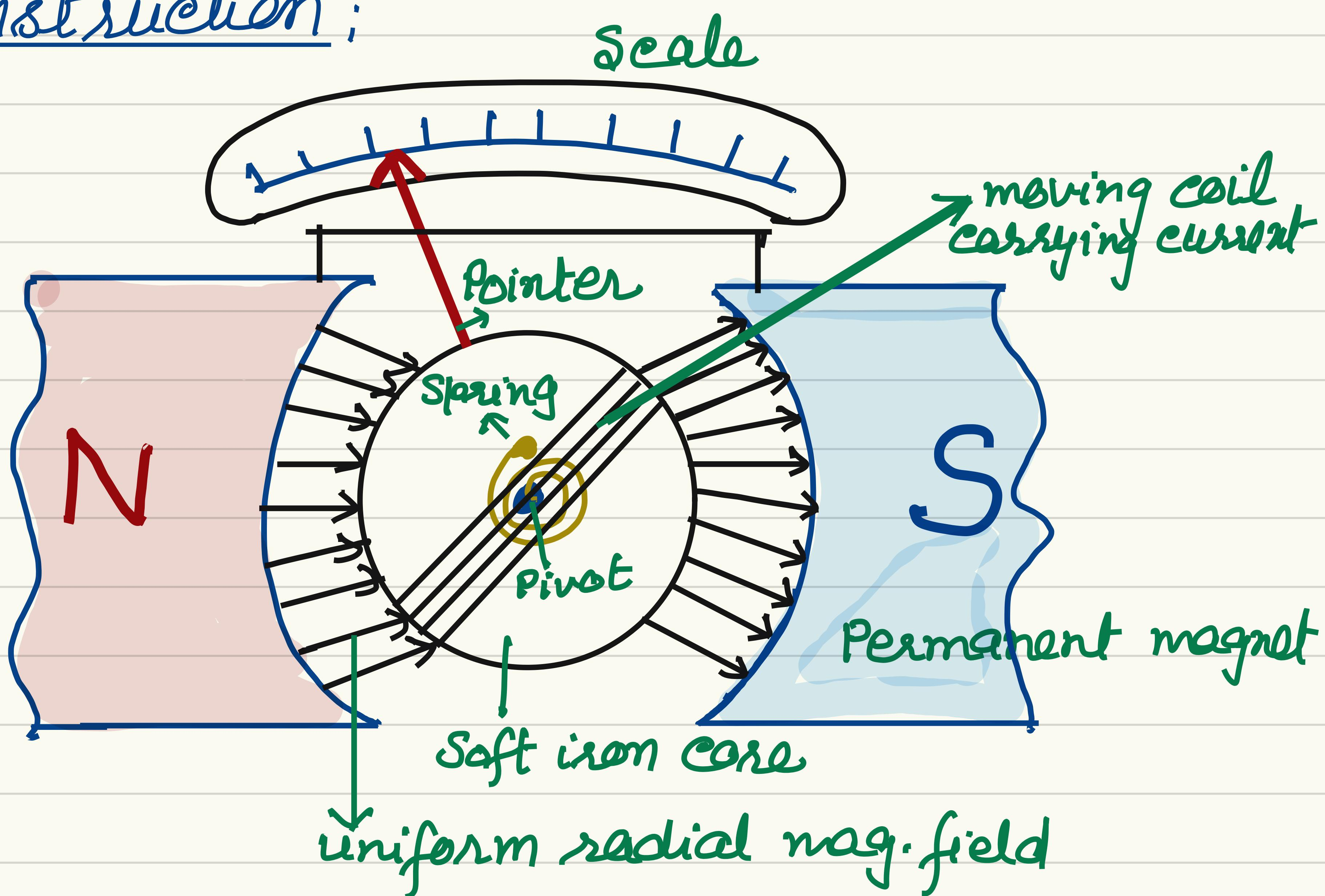
A Weston galvanometer consists of a rectangular coil of fine insulated copper wire wound on a light non magnetic (Al) frame. The two ends of circle of this frame are pivoted by two jewelled bearings. The motion is controlled by a pair of hair springs of phosphor bronze. The spring provided restoring torque.
