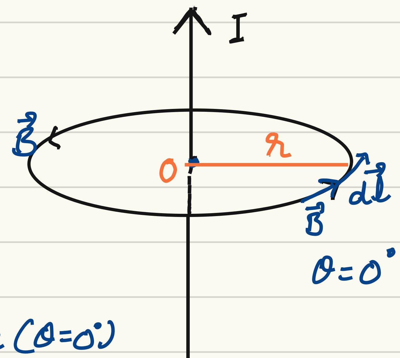
here  $\vec{B}$  and  $d\vec{l}$  are in same direction ( $\theta=0^\circ$ )
