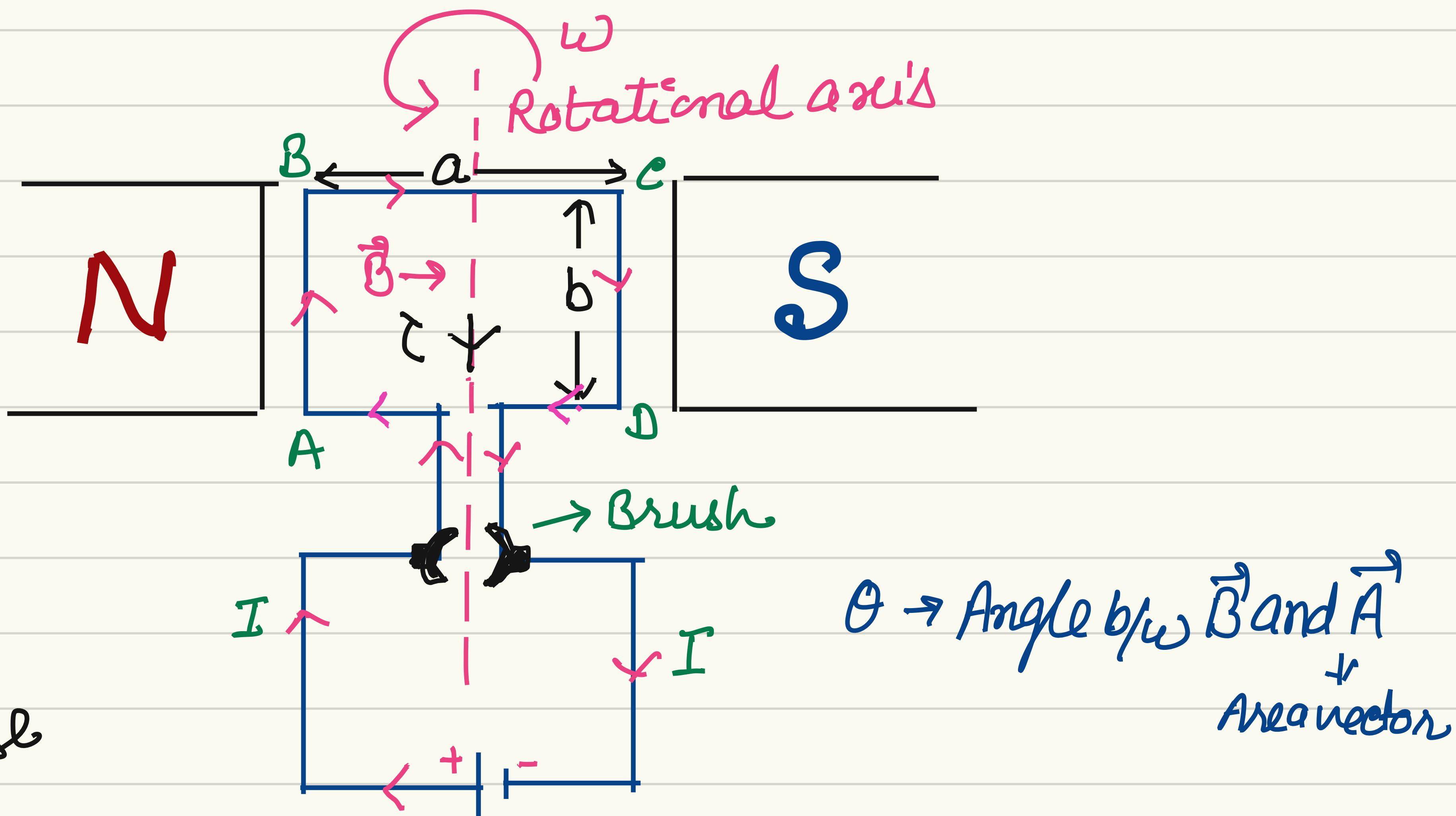
Case I When mag. field is in the plane of the loop. ( $\theta = 90^\circ$ )
