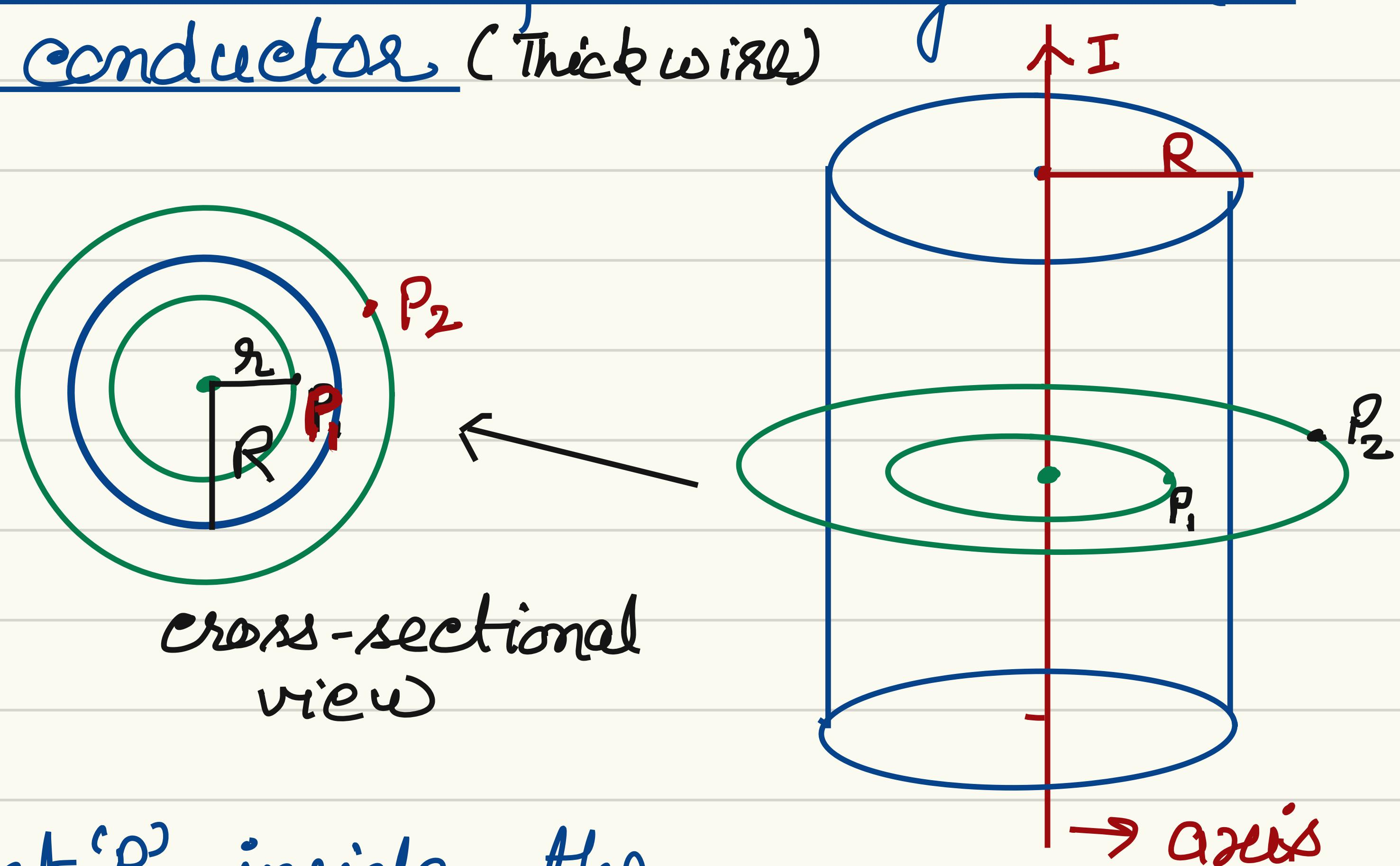
(i) For a point 'P<sub>1</sub>' inside the cylinder ( $r < R$ )
